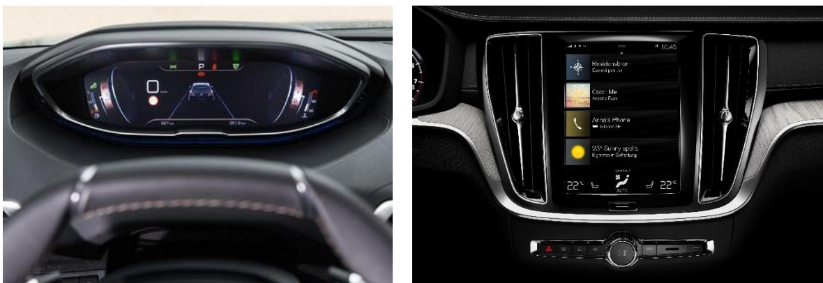
Figure 5.4: Built-in HMI example. The left picture shows a display directly in front of the driver, while the right picture depicts a display centered between driver and co-driver, where driving instructions can be depicted on both.
