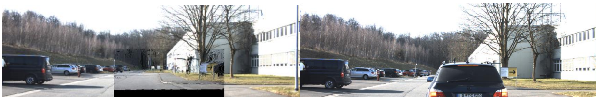
Figure 3.9: HMI of the see-through system in the rear car. In the left picture the see-through video overlay is activated and in the right picture the overlay is deactivated.
