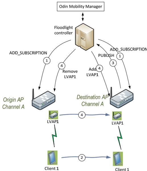
Fig. 2. Scheme of a handover with Odin
