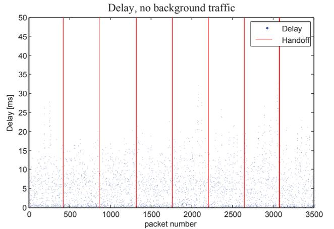
Fig. 3. Delay *Quake 3* packets when no background traffic is present
