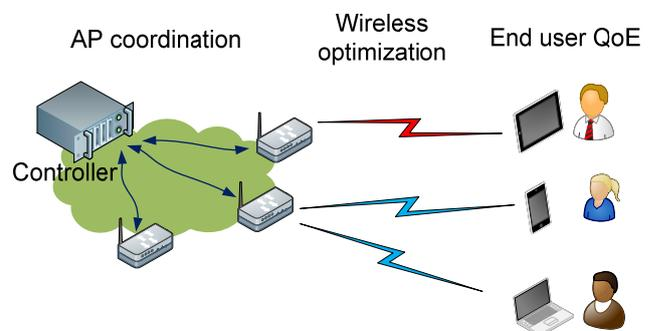
Fig. 1. Basic scheme of the smart APs architecture
